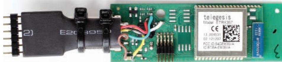
■ Photo 5. Here is the Combined Interface device after its embedded development mode modification. The Digilent six-pin connector cable is a female-to-female type. The Combined Interface device embedded interface must be male. The female-to-male conversion is done using an extended male header.
